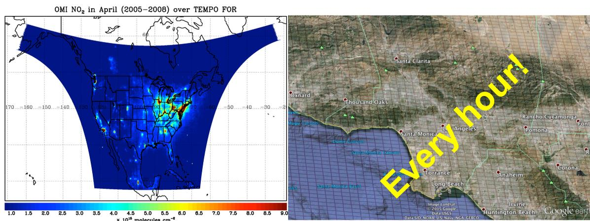
Figure 1. Left: The TEMPO field of regard (FOR), as swept hourly (illustrated using OMI NO<sub>2</sub> data). Right: The resulting hourly coverage over the greater Los Angeles region.
