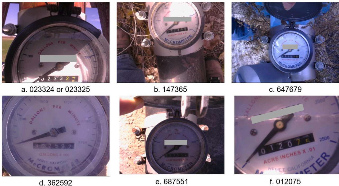
Fig. 6. . Examples of successfully recognized accumulative water flow (digits in black box on the dial) in the flow meter images. Caption under each image shows recognized readings from the proposed algorithm.
