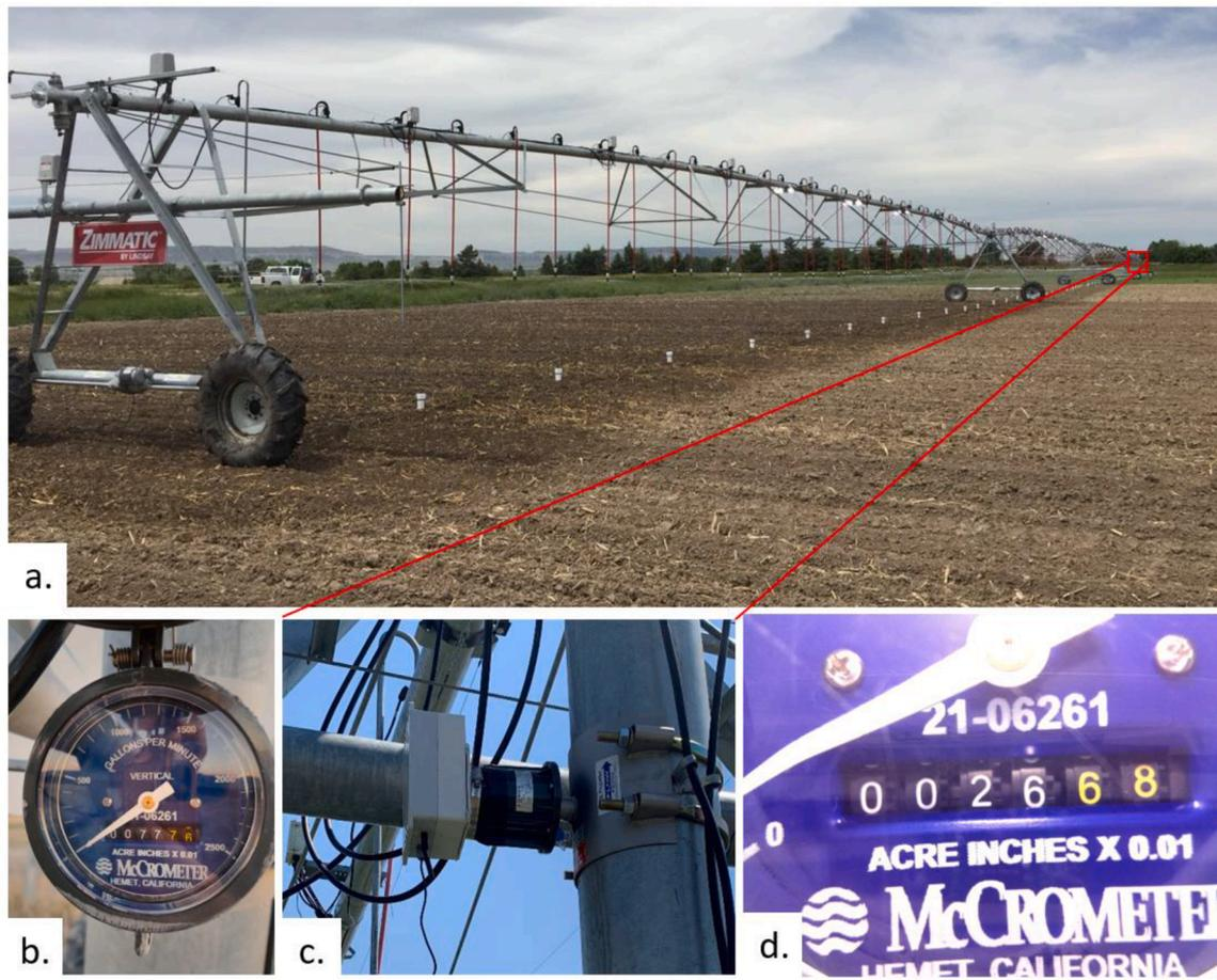
**Fig. 5.** a. a linear-move sprinkler irrigation system at Panhandle Research and Extension Center, University of Nebraska-Lincoln, Scottsbluff, NE, USA. b. an analog-style vertical flow meter. c. an AI-FlowCAM mounted on top of the flow meter. d. an image taken by AI-FlowCAM.
