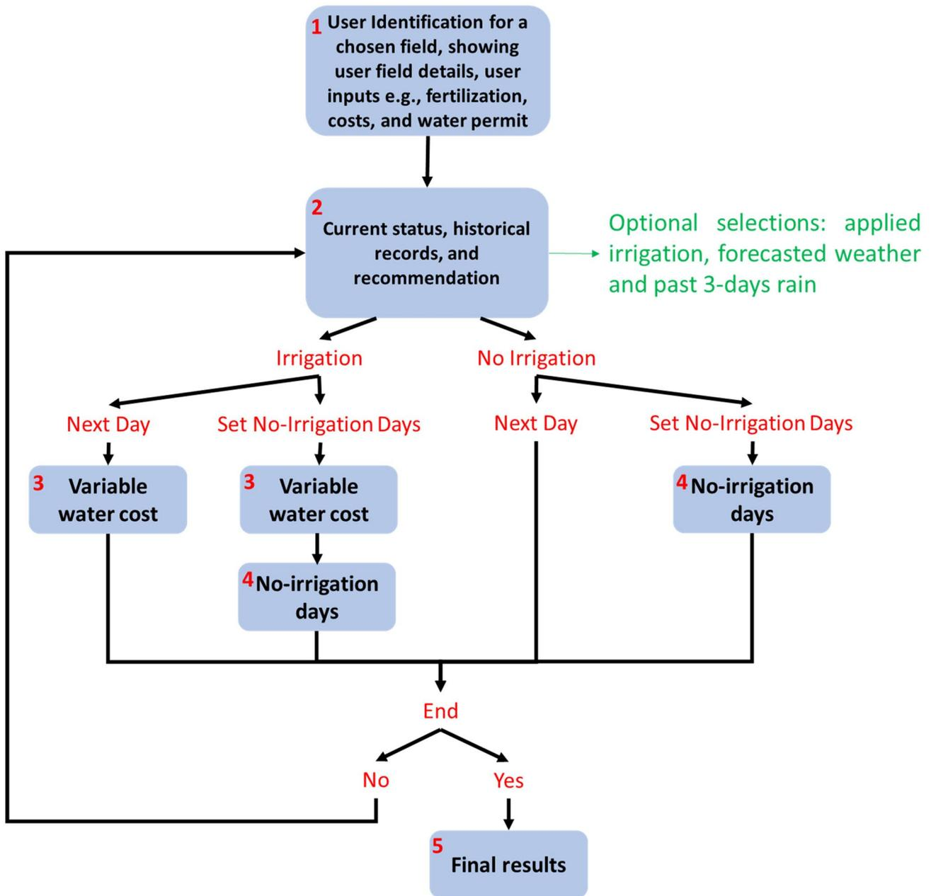
**Figure 3.** The flowchart of the Graphical User Interface designed for the human-machine interaction. The window number at each stage is shown in bold red.
