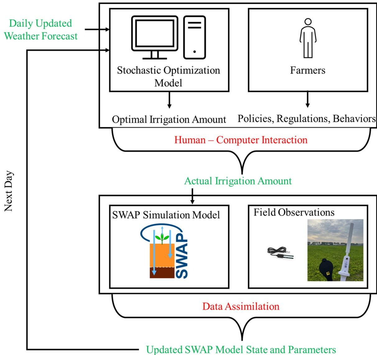
**Figure 1.** Overall framework of RTSIT composed of stochastic optimization, soil-crop simulation, data assimilation, and human-computer interaction.
