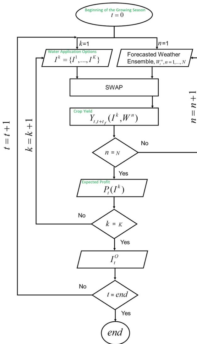
**Figure 2.** The simulation-optimization framework. The framework is composed of three loops with time ( $t$ , crossing the irrigation season), weather forecast scenarios ( $n$ ), and water applications ( $k$ ).
